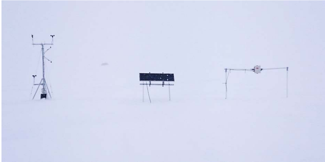
Figure 5-6: The mobile weather station (left) and the spectral radiance station (right) with the solar panel (middle) in Valdresflya spring 2015.
